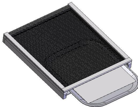
Fig 2. Screened bottom board showing the position of screws in the ends of the 7/8" parts
